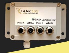
The '2 +2' models differ from the '4' model in that the former controls 2 solenoid irrigation valves and 2 pressure sensors while the latter controls 4 solenoid irrigation valves without the pressure sensors for flow verification.
